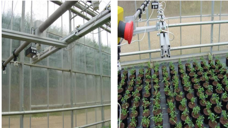
Figure. 7.19. The thermopile system with remote monitoring mounted on a gantry watering system.
