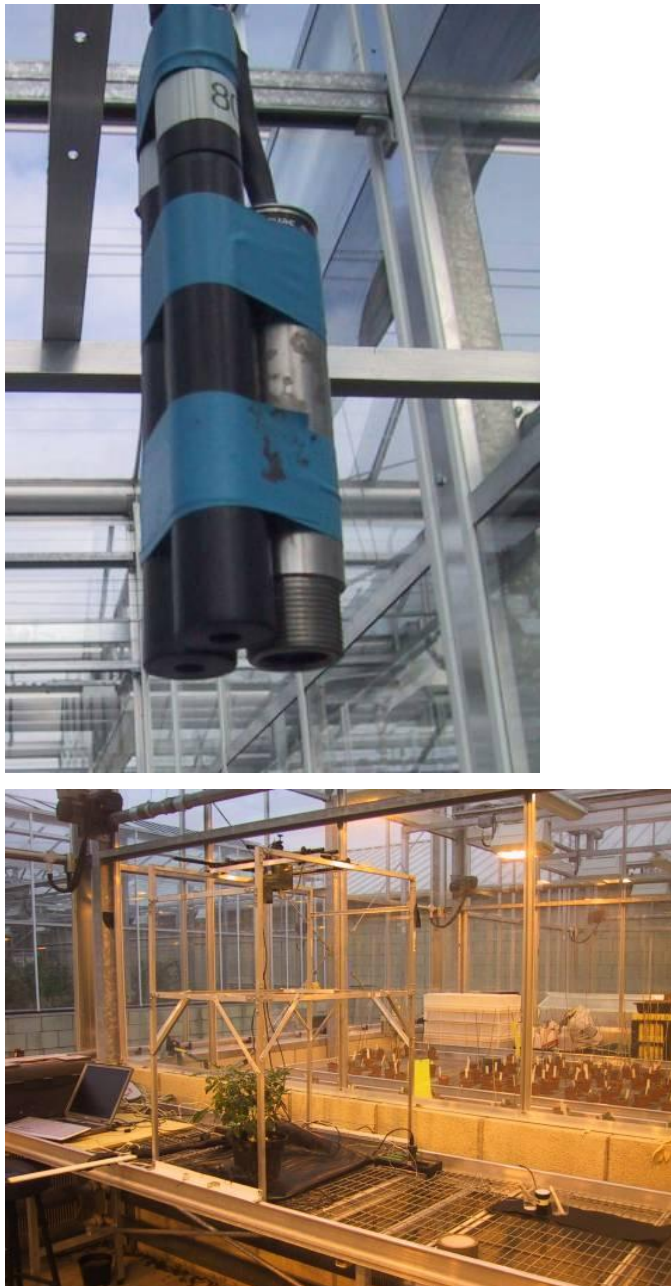
Figure 7.4. Left - Three sensor cluster with thermal sensor (8-14 \mu\text{m} ), red (650 nm) and NIR (800 nm) sensors. Right - Experimental setup.
