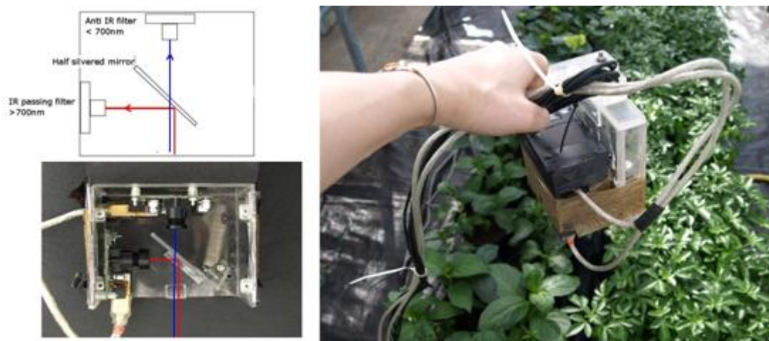
Figure 7.3. Left - Twin webcam NDVI sensor construction. Right - Handheld scanner NDVI sensor combined with Calex temperature sensor.
