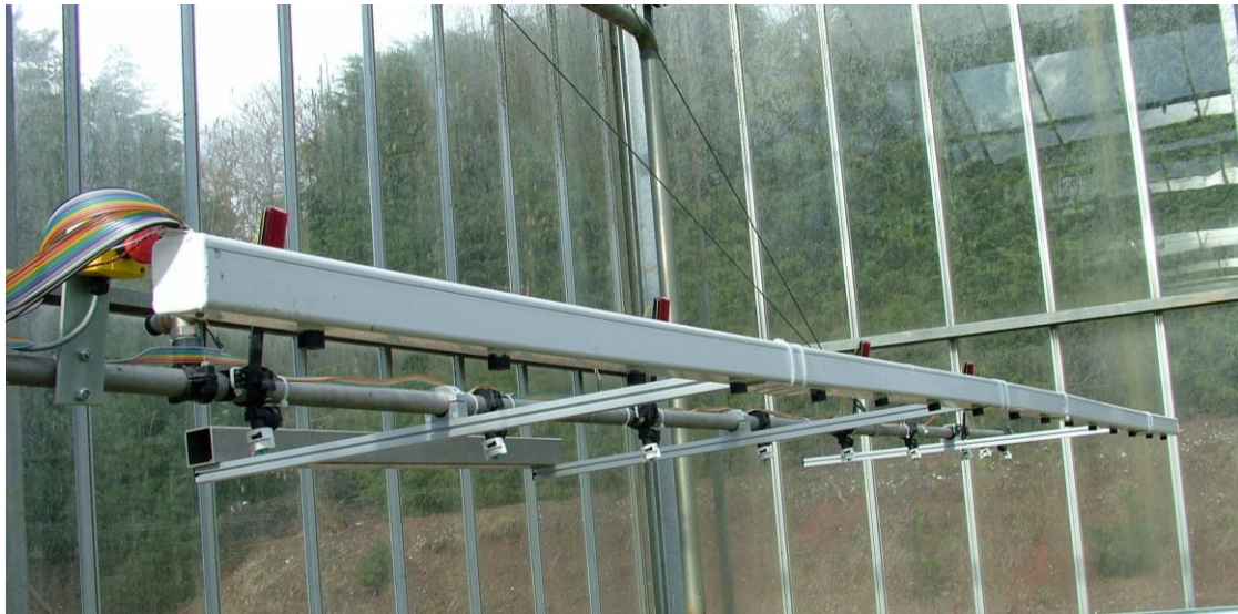
G.S. Figure 9. A temperature sensing boom containing 16 thermopile sensors mounted in front of one arm of the irrigation boom on a Denton Automation gantry.
