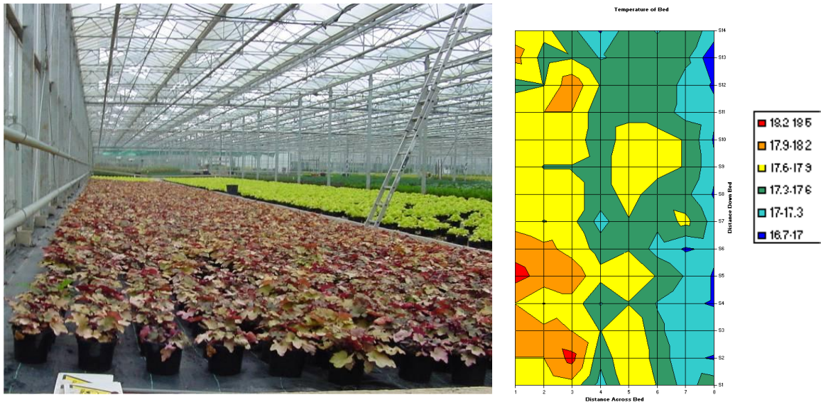
G.S. Figure 10. Results from a scan of Heuchera plants on a sloping bed using the gantry mounted thermopile array. It shows dryer / warmer areas at the top of the slope (yellow / orange) and wetter / cooler areas at the bottom of the slope (green / blue).
