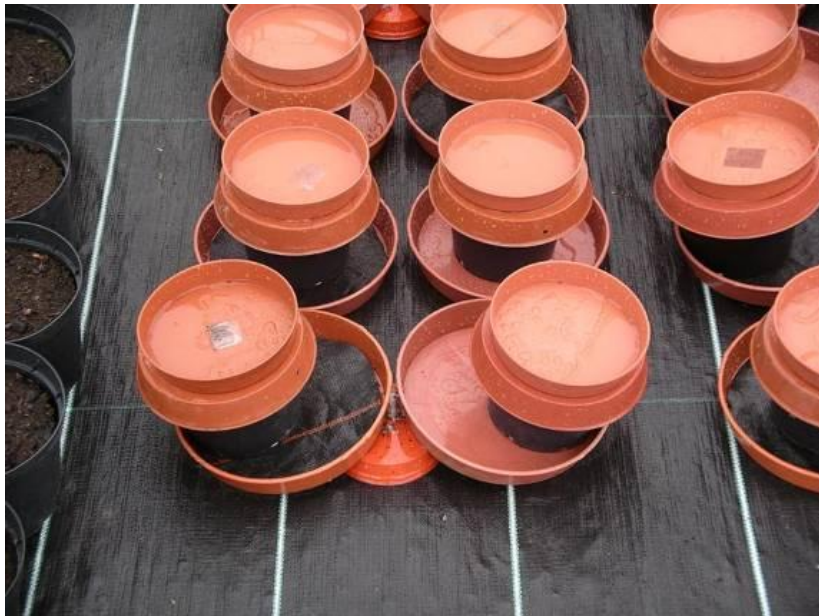
Figure 1.8. Experiment with standard water absorbency pots to determine the effects of Mypex and a sloping surface on moving water across the surface towards the pot. Puddles of free water are visible in the saucers which are horizontal and without a Mypex disc.
